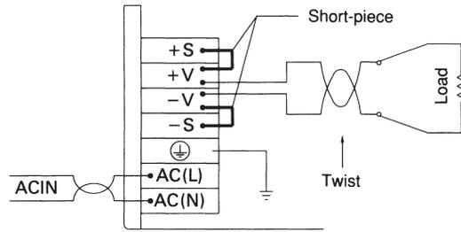
(2)When using remote sensing function
