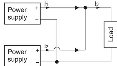
■Even a slight difference in output voltage can affect the balance between the values of I1 and I2.
