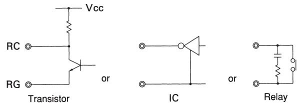
When RC terminal is "Low" level, fan out current is 3mA typ. When Vcc is applied, use  $5V \leq V_{cc} \leq 12V$ . When remote ON/OFF function is not used, please short between RC and RG terminals.
