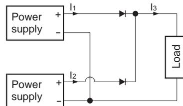
■ Even a slight difference in output voltage can affect the balance between the values of I<sub>1</sub> and I<sub>2</sub>.
