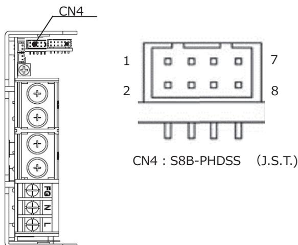
Fig 2.1 Example of option -I4 (AEA600F)
