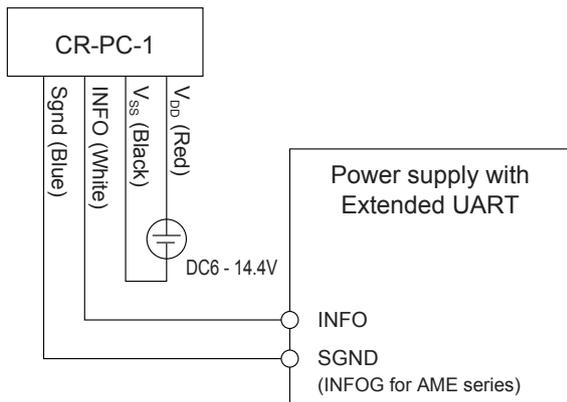
(3) Connecting a CR-PC-1 to multiple power supplies with Extended UART
