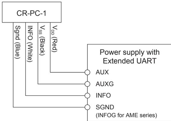
(2) For power supplies with Extended UART which do not have AUX (12V) power.
